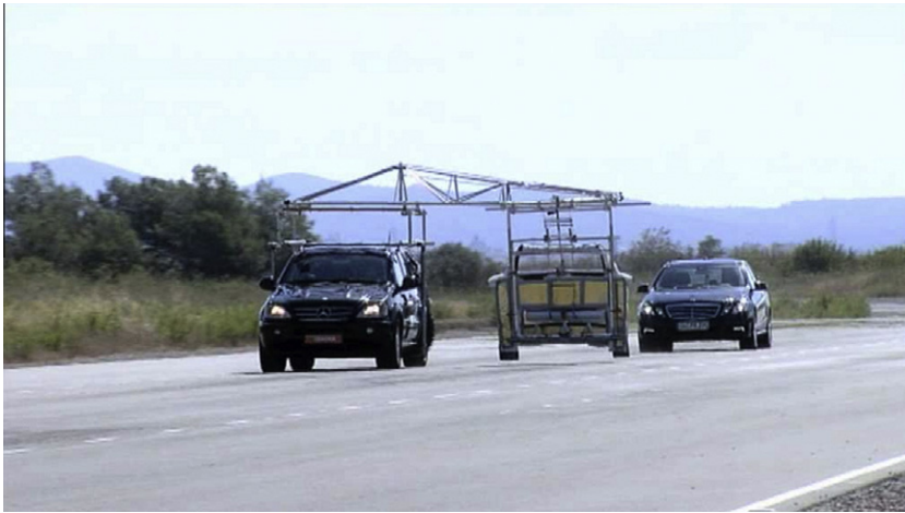
Fig. 8. EEBL testing vehicles with foam platform at IDIADA's proving ground.
